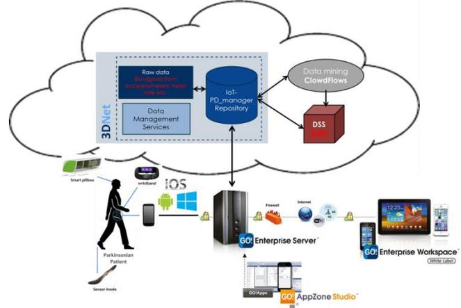
Fig. 1. The overall PD\_manager architecture
